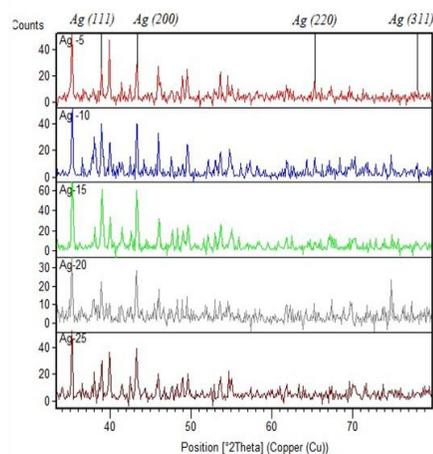
Fig.2: XRD diffraction of Ag with different concentration of reducing agent
