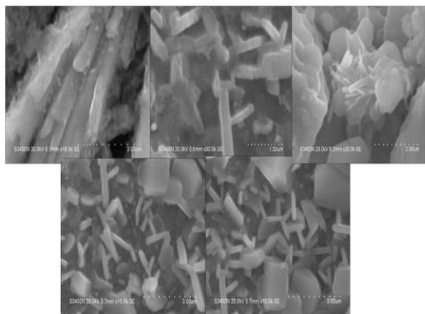
**Fig.4: SEM Images of all silver nanoparticle samples.**
