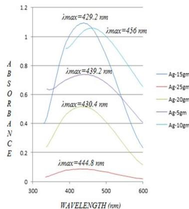
Fig.1: UV absorbance of silver nanoparticles obtained from 5 different concentration of papaya extract
