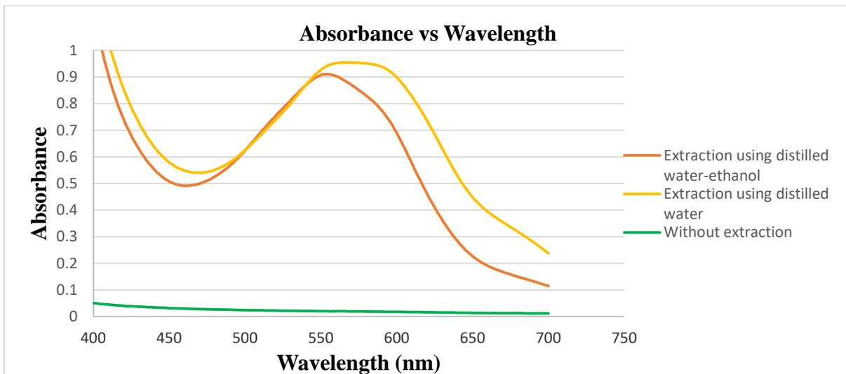
Fig. 2 UV-vis spectra of pH indicator films with and without purple cabbage extract
