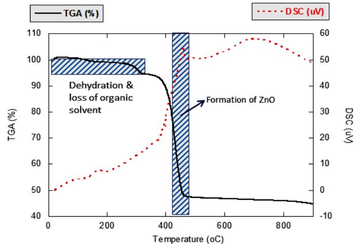
**Fig. 2** DSC/TGA thermograms of the electrospun ZnO fibers
