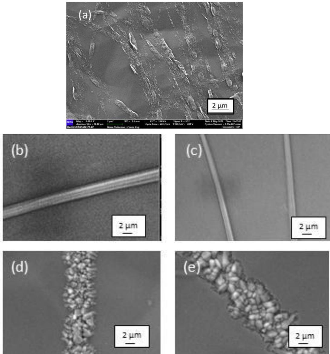
**Fig. 4** FESEM images of electrospun ZnO fibers calcined at (a) 400 °C, (b) 500 °C, (c) 600 °C, (d) 700 °C and (e) 800 °C
