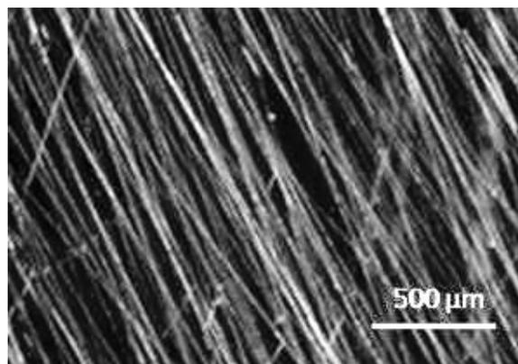
**Fig. 1** Optical image of the aligned electrospun PVP/zinc acetate fibers
