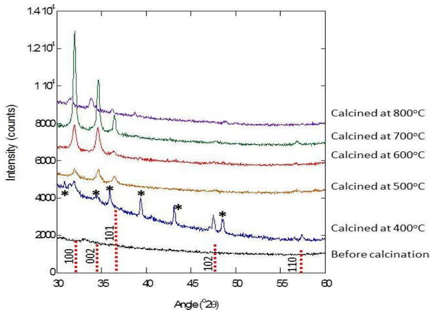
**Fig. 3** Comparison of X-ray diffractograms of the electrospun ZnO fibers calcined at different temperatures. (The dotted stick pattern represents the peak positions of ZnO taken from JCPDS No: 00-001-1136 and \* represents the peak positions of zinc acetate from JCPDS No.00-001-0089)
