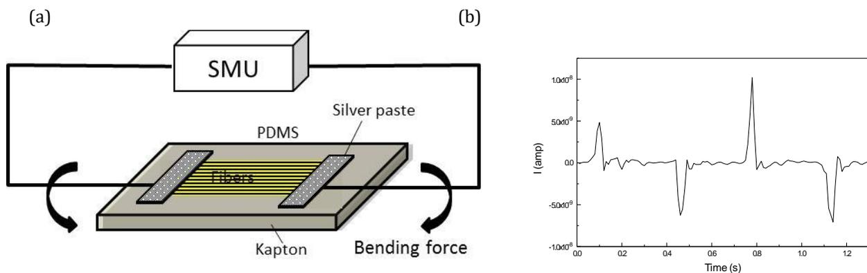
**Fig 5** (a) Schematics of a ZnO piezo generator and (b) The current pulse produced when the fibers were bent and released
