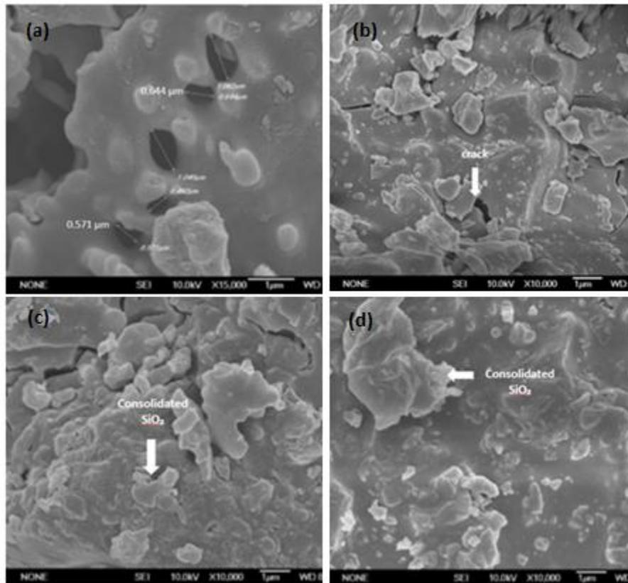
**Fig. 2** FESEM images of fabricated silica ceramic membrane at different calcination temperature, (a) ceramic support; (b) 400 °C, (c) 500 °C and (d) 600 °C
