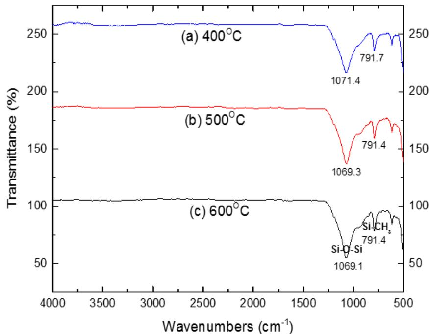
**Fig. 3** FTIR adsorption spectra of prepared ceramic membranes at different calcination temperature
