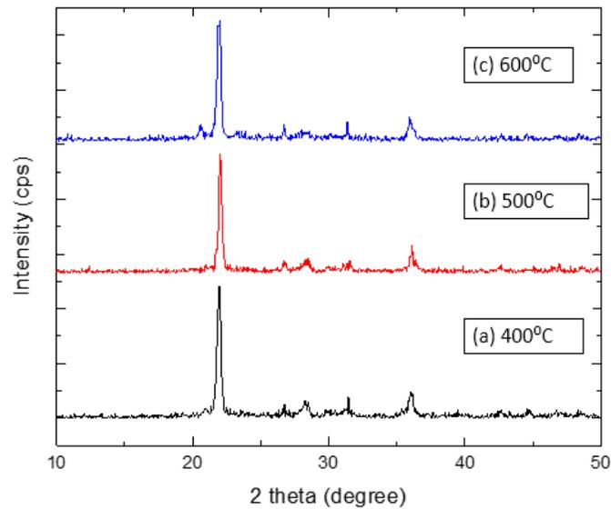
**Fig. 1** XRD pattern of fabricated silica ceramic membrane at different calcination temperature, (a) 400 °C, (b) 500 °C and (c) 600 °C
