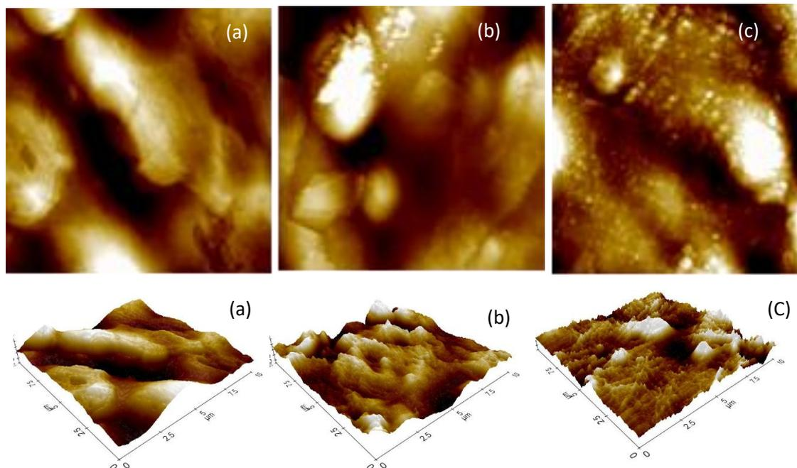
**Fig. 2** AFM topographic images of (a) PP, (b) PP/K 3%, and (c) PP/K 5 %
