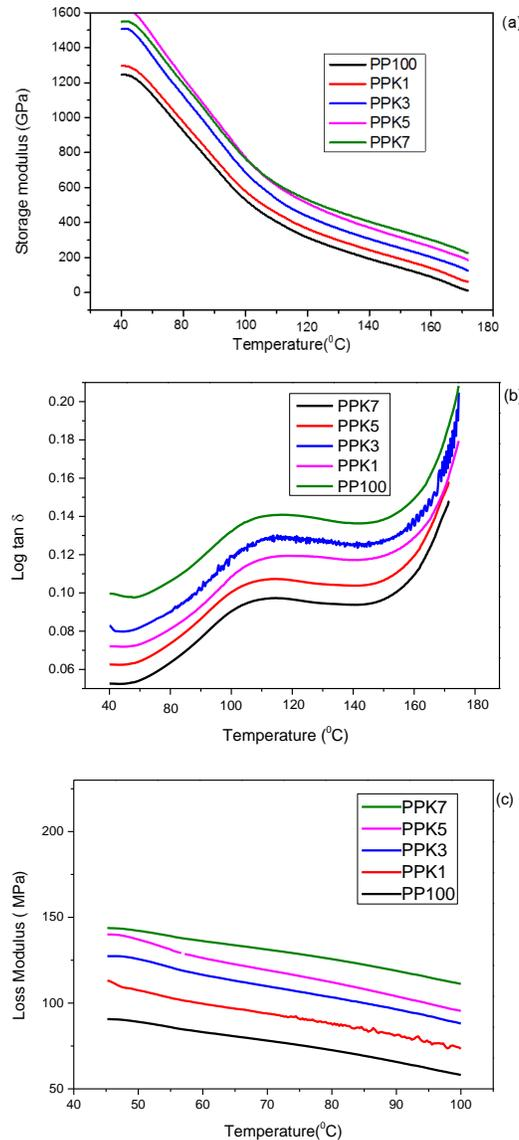
**Fig. 1** DMA spectra of pristine PP and PP/K nanocomposites (a) Storage modulus, (b) Tan  $\delta$  and (c) Loss modulus
