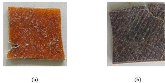
**Fig. 4** The appearance of (a) LDPE/TPS and (b) LDPE/TPS/10 wt.% BPF samples after subjected to soil burial test
