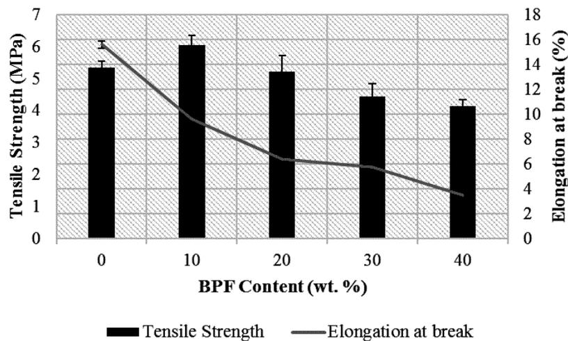
**Fig. 1** Effect of banana peel fiber content on the tensile strength and elongation at break of LDPE/DSS blends
