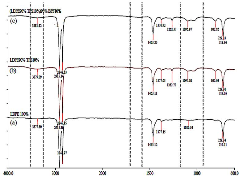
**Fig. 3** FTIR spectra of the composites of (a) LDPE, (b) LDPE/TPS and (c) LDPE/TPS/10 wt.% BPF
