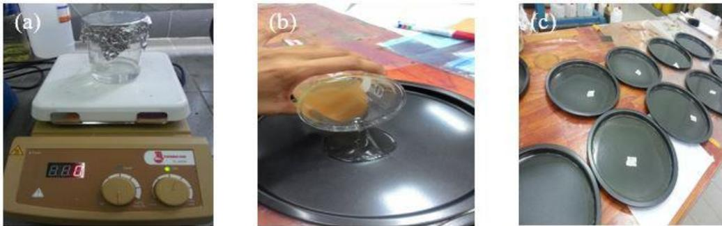
**Fig. 1** The sample preparation of PLA/DSF biocomposite films (a) stirred process with magnetic agitation on hot plate; (b) poured the sample onto flat mould and (c) left the samples for drying process
