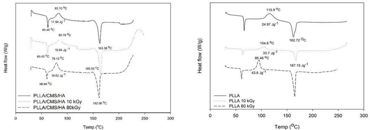
**Fig. 3** DSC thermogram of irradiated and non-irradiated samples, (a) PLLA and (b) PLLA/CMS/nHA at 10 and 80kGy
