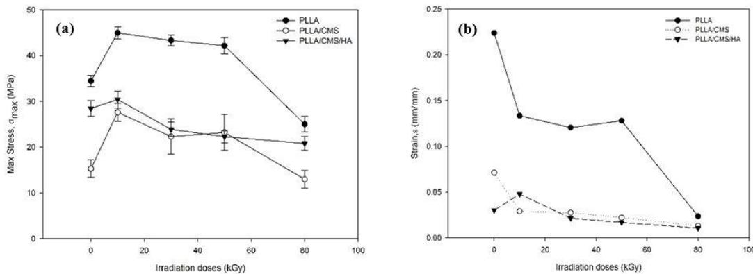
**Fig. 2** (a) The ultimate strength and (b) Strain of PLLA, PLLA/CMS and PLLA/CMS/HA of both non-irradiated and irradiated at 10 and 80kGy
