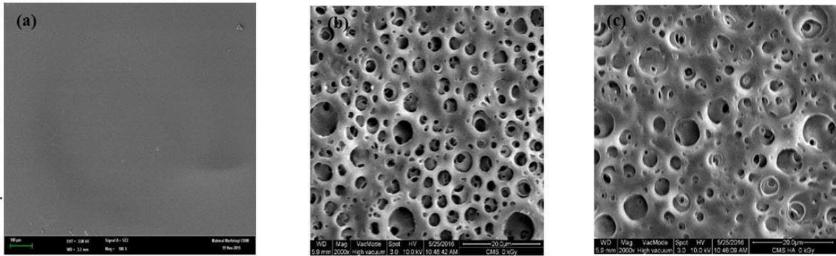
**Fig 1** The SEM micrograph of (a) PLLA, (b) PLLA/CMS and (c) PLLA/CMS/HA of non-Irradiated sample produced by casting evaporation method.
