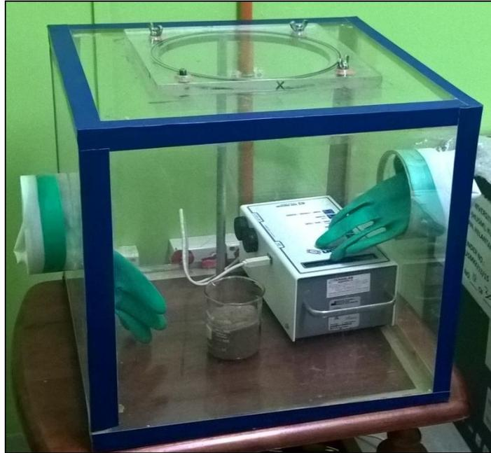
**Fig. 2** Radon Sentinel 1030 monitor was used to determine  $^{222}\text{Rn}$  concentrations level emanated from collected soil samples
