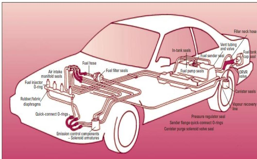
Fig. 1 Non-metal automotive components in fuel system [8]
