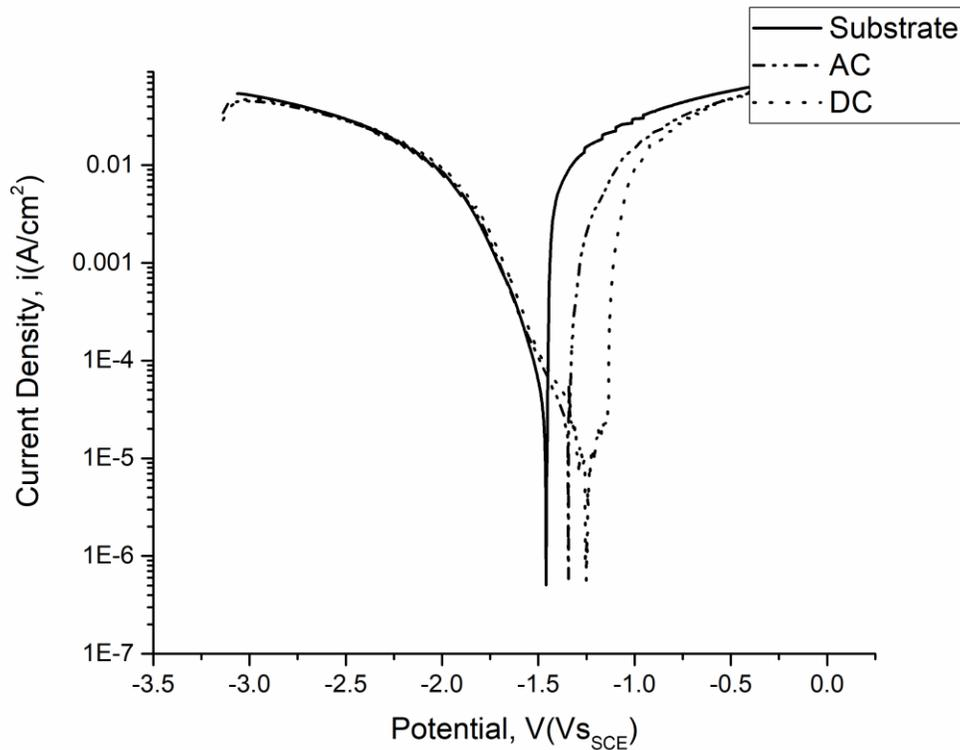
**Fig. 1** Potentiodynamic polarization curves for the anodized specimens both AC and DC at 30 V
