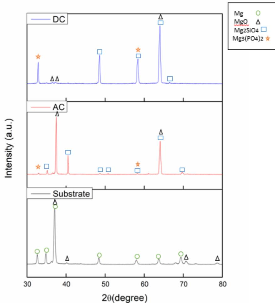
Fig. 3 XRD pattern for anodized sample
