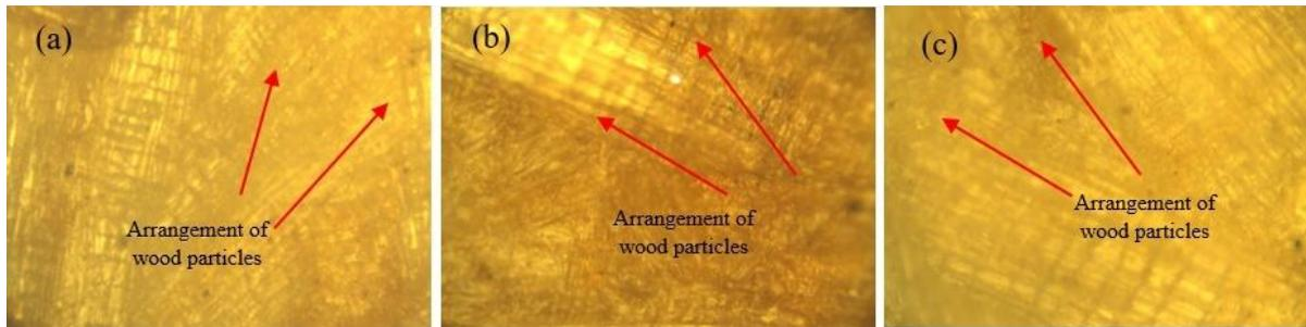
**Fig. 2** Surface morphology panel NC species of (a) 8%, (b) 10%, and (c) 12% of UF
