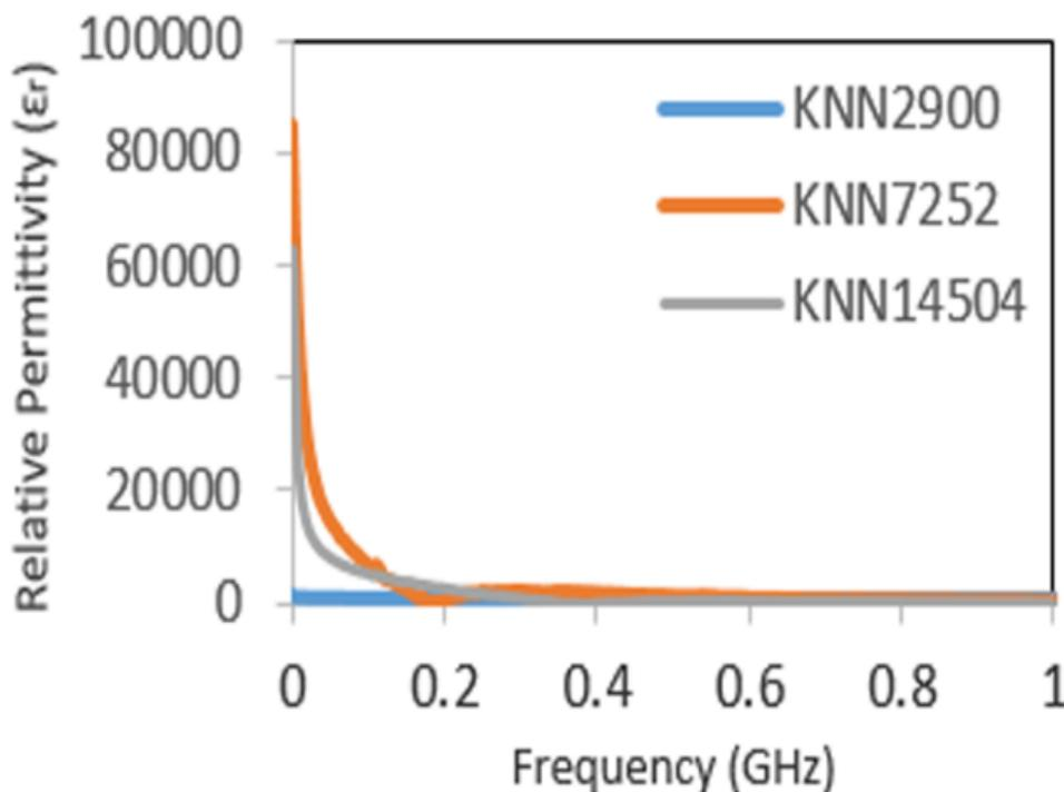
**Fig. 3** The relative permittivity of KNN samples after applied 3 different pressure during sintering process (2900, 5257 and 14504 psi)
