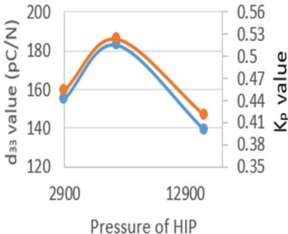
**Fig. 4** The variations of piezoelectric properties ( $d_{33}$  and  $k_p$  value) of KNN samples after being applied 3 different pressure during sintering process by HIP technique (2900, 5257 and 14504 psi)
