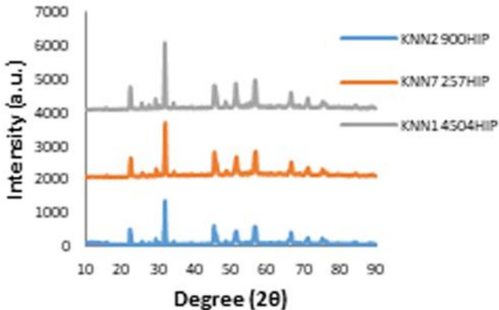
Fig.1 The XRD pattern of the KKN samples after prepared under different sintering pressure of
