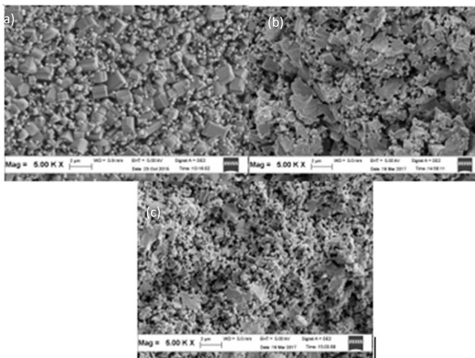
Fig. 2 The FESEM micrograph of KNN samples after applied 3 different pressure during sintering process by HIP (a) 2900, (b) 5257 and (c)14504 psi
