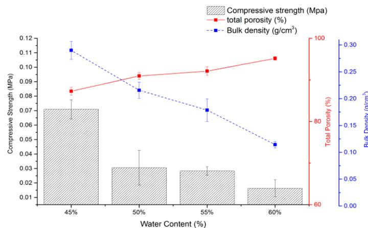
**Fig. 3** The compressive strength of the samples with the bulk density accordingly
