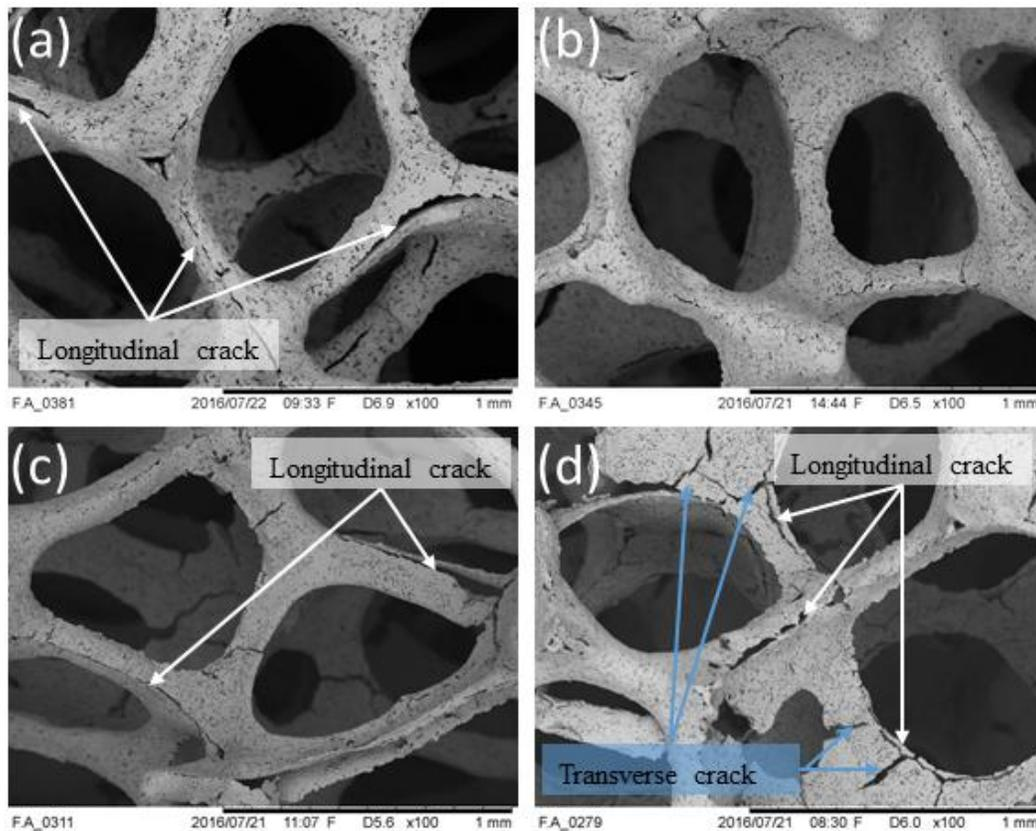
**Fig. 2** The SEM micrographic of sintered porous cordierite prepared by (a) 45, (b) 50%, (c) 55% and (d) 60 % water content slurry
