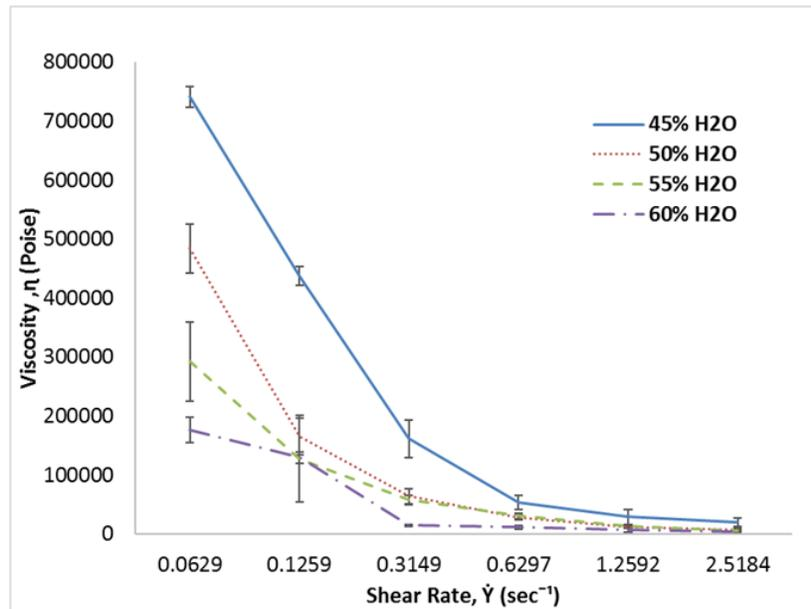
**Fig. 1** Viscosity profile of MAS slurries with different water content respectively
