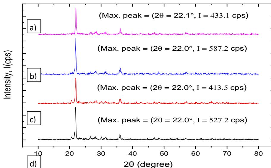
**Fig. 2** XRD pattern for fabricated silica ceramic membrane with different silica sol molar ratio (a) R=4.7, (b) R=4, (c) R=3, and (d) R=2
