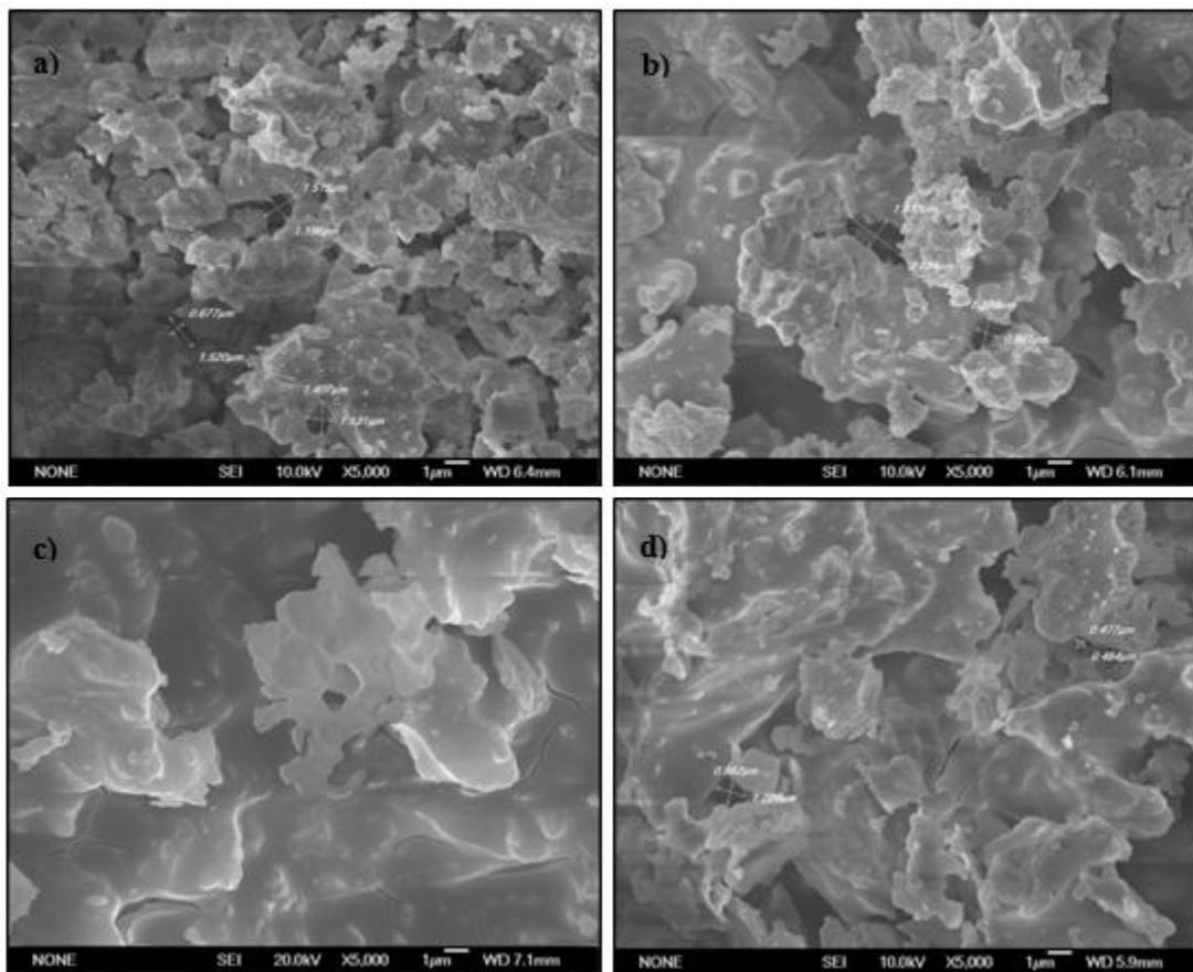
**Fig.3** FESEM images of fabricated silica ceramic membrane at different silica sol molar ratio (a) R=4.7, (b) R=4, (c) R=3, and (d) R=2
