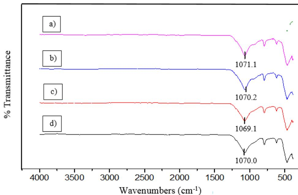
Fig. 5 FTIR result of fabricated silica ceramic membrane at different silica sol molar ratio (a) R=4.7, (b) R=4, (c) R=3, and (d) R=2
