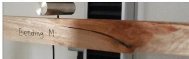
Fig. 6 The crack at the lower parts of the specimen that explains the wood fibres fails due to tension stress during bending
