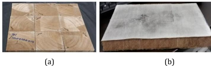
**Fig.1** (a) Mahang core of sandwich composite and (b) Sandwich composite with fibreglass face skin and mahang core
