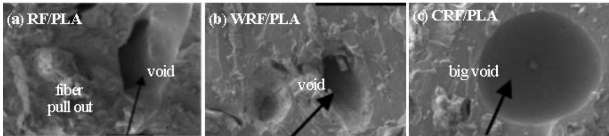
**Fig. 4** Morphological of failure structures of the composite boards, (a) RF/PLA, (b) WRF/PLA and (c) CRF/PLA
