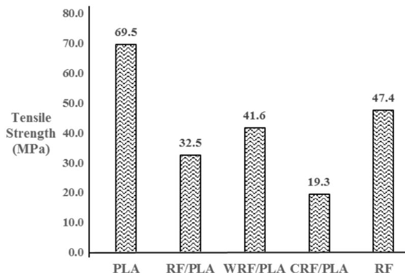
**Fig. 3** The graph of tensile strength for PLA, composite boards and rattan fibers
