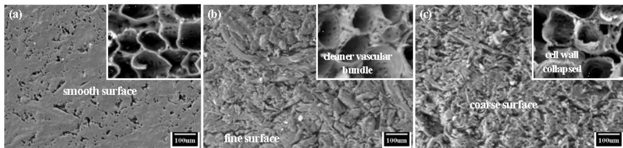
**Fig. 5** Morphological structure of surfaces of composite boards, with the fiber structures under 1000x magnification (in inserted pictures). From left: (a) RF/PLA, (b) WRF/PLA, (c) CRF/PLA
