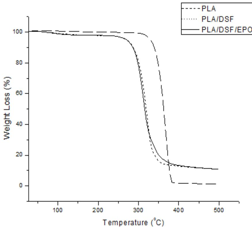
**Fig. 1** TGA curves for PLA, PLA/DSF and PLA/DSF/EPO biocomposites
