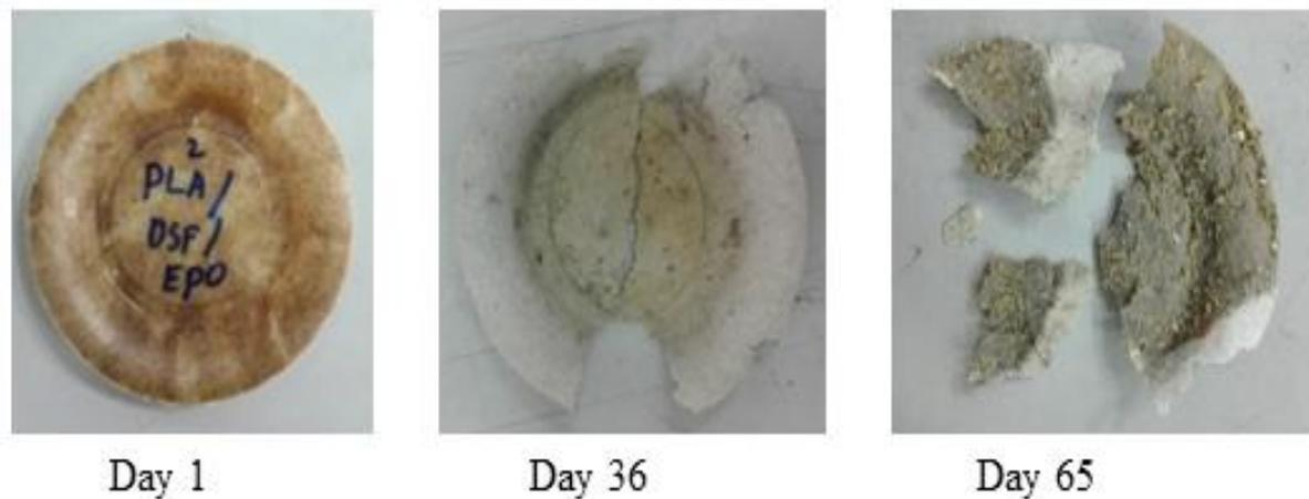
Fig. 2 Degradation time of PLA/DSF/EPO
