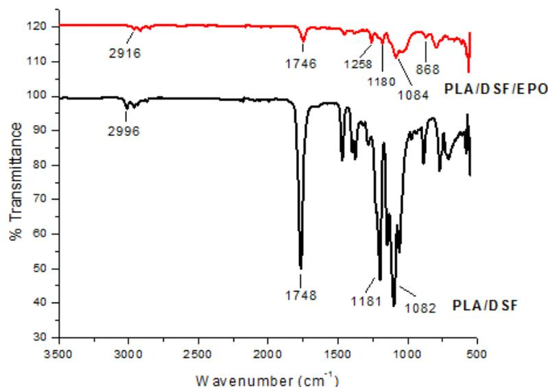
Fig. 3 FTIR spectrum of PLA/DSF/EPO
