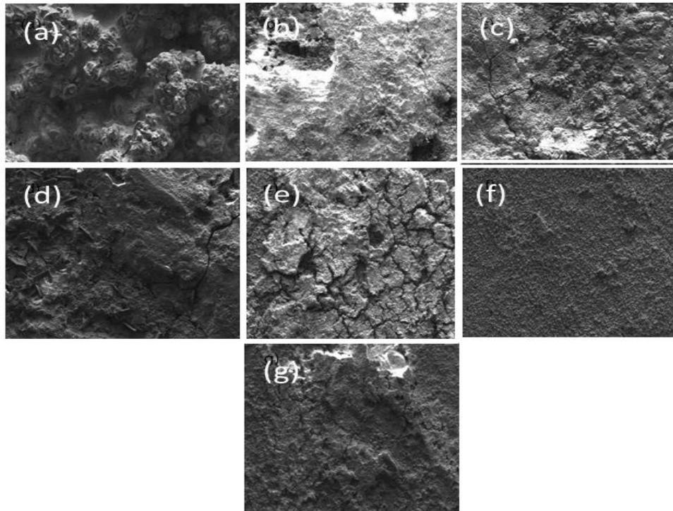
**Fig. 2** Effect of pH on the surface morphology of Cu-Sn-Zn alloy coating at pH (a) 1.0, (b) 3.0, (c) 5.0, (d) 7.0, (e) 9.0, (f) 11.0 and (g) 14.0 deposited at 15 mA/mm<sup>2</sup>
