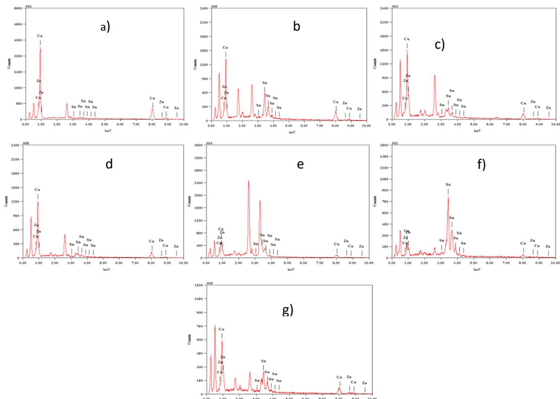
**Fig. 3** EDS spectrum of Cu-Sn-Zn alloy coating at pH (a) 1.0, (b) 3.0, (c) 5.0, (d) 7.0, (e) 9.0, (f) 11.0 and (g) 14.0 deposited at 15 mA/mm<sup>2</sup>
