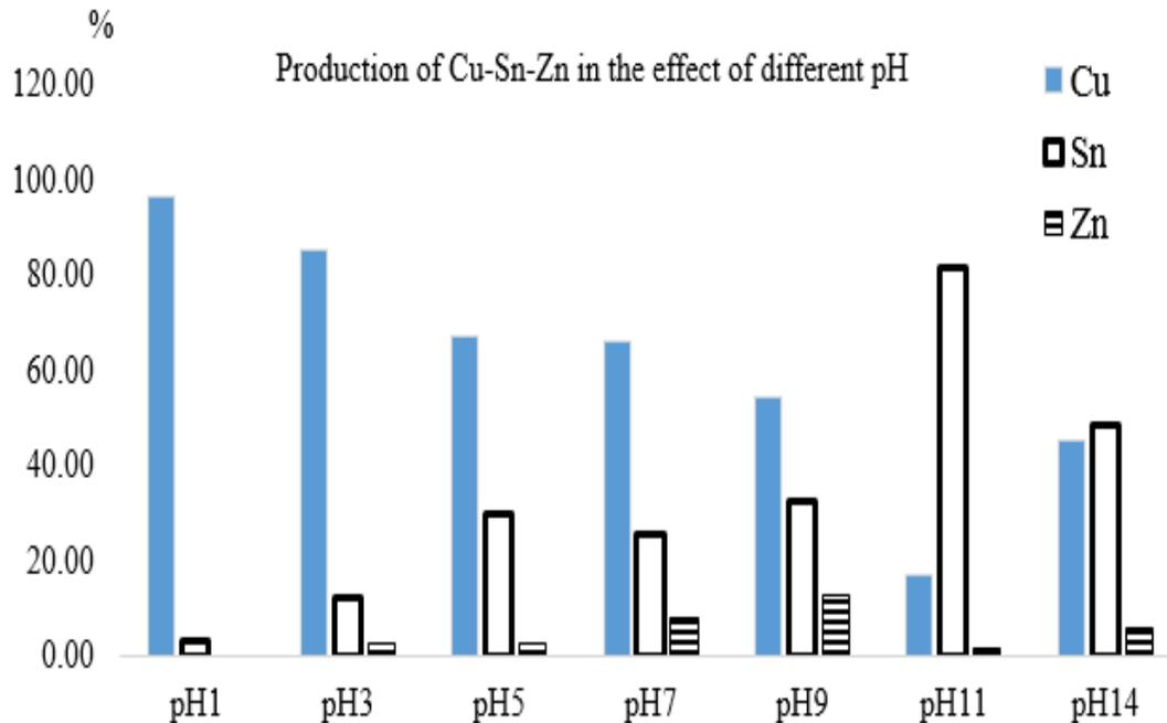
**Fig. 1** Production of Cu, Sn and Zn in the effect of different pH
