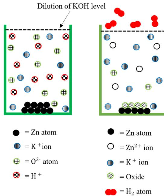
**Fig. 4** Illustration of Zn reaction in KOH solution
