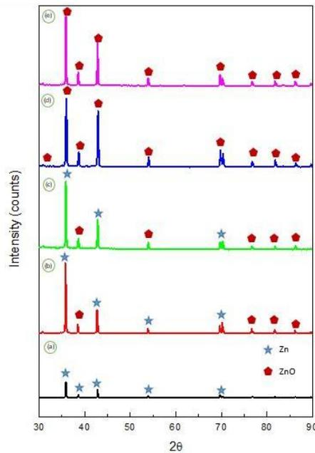
**Fig. 3** Comparison peak analysis for XRD of (a) Zn commercial and Zn after reaction with (b) 2, (c) 4, (d) 6 and (e) 8 M of KOH
