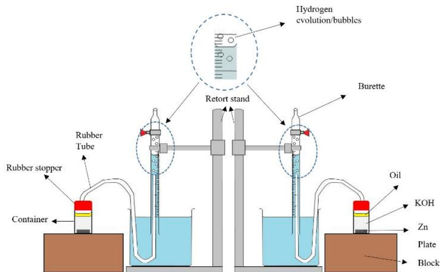
**Fig. 1** Schematic diagram of volumetric measurement setup
