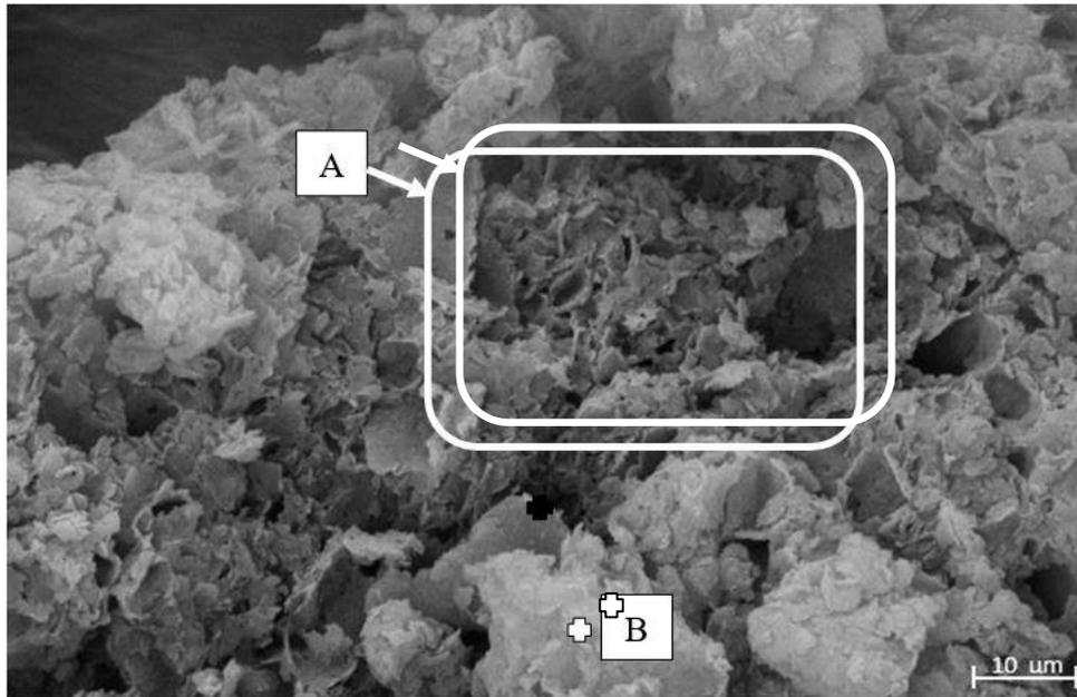
**Fig. 1** SEM image of 2D MXene  $\text{Ti}_3\text{C}_2$  after etching process in 49% HF solution
