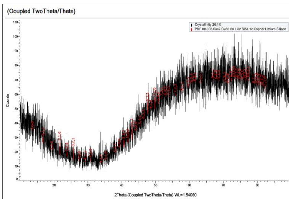
**Fig.1.** X-ray diffraction pattern for the banana peel waste sample
