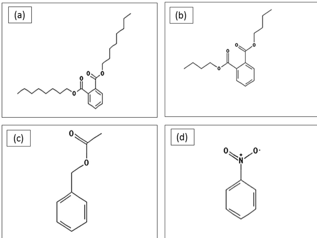
Fig. 3 The structure of plasticizer (a) Dioctyl phthalate (DOP), (b) Dibutyl phthalate (DBP), (c) Benzyl acetate (BA) and (d) Nitrobenzene (NB)
