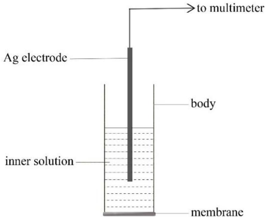
**Fig. 1** Ion Selective Electrode (ISE)
