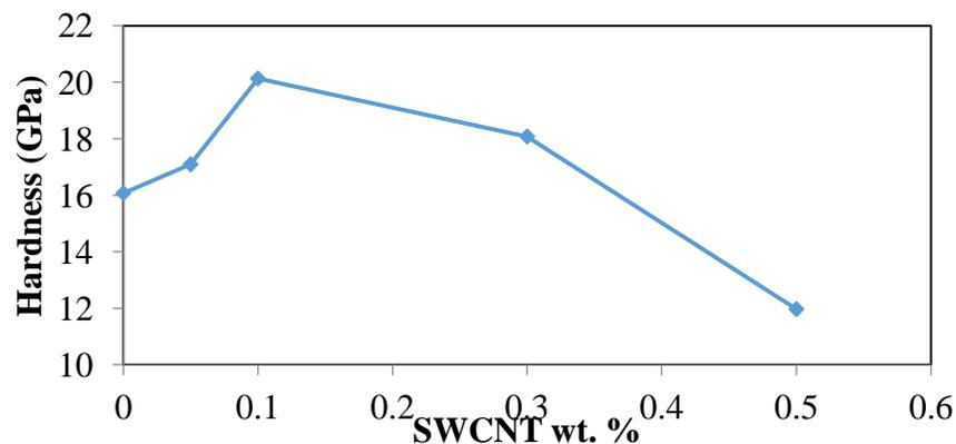
Fig. 6. Hardness of  $Al_2O_3$  with different composition of SWCNT
