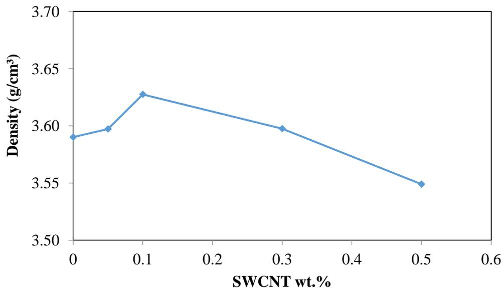
**Fig.4.** Density of  $\text{Al}_2\text{O}_3$  with different composition of SWCNT
