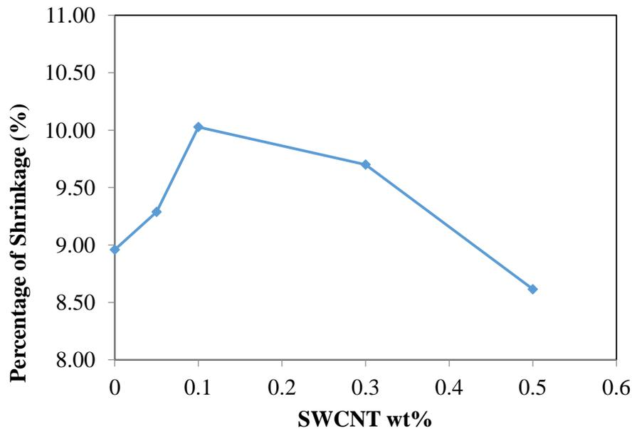
Fig. 5. Percentage of shrinkage of  $Al_2O_3$  with composition of SWCNT
