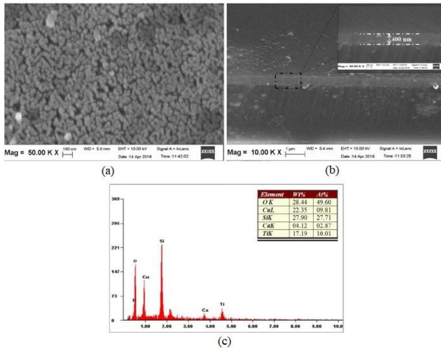
**Fig. 3** SEM micrographs of CCTO thin layer (a) topside, (b) cross section and (c) EDX analysis
