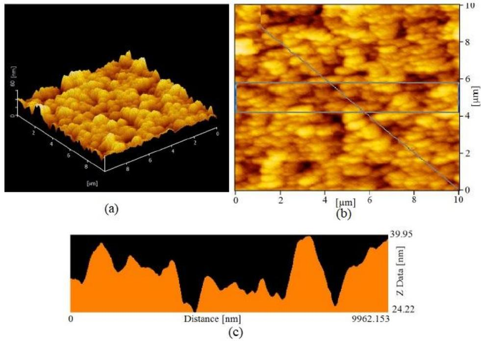
**Fig. 2.** Atomic force micrographs of CCTO thin layer (a) 3D image, (b) 2D image and (c) the corresponding average profile line
