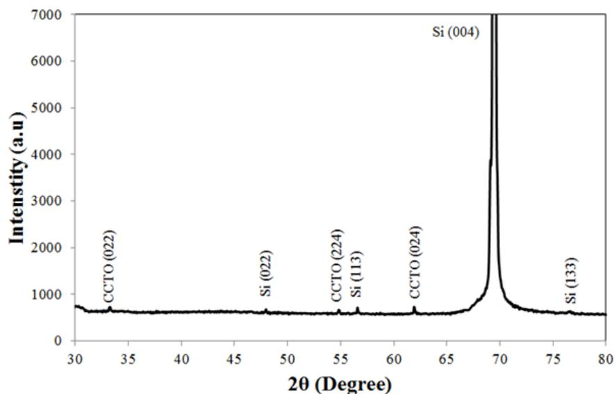
**Fig. 1** XRD patterns of the sputtered CCTO thin layer on silicon wafer
